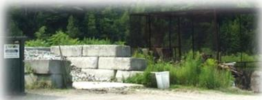
Glass aggregate (bottles, window glass and ceramics) is collected in a bunker constructed from concrete blocks. This is crushed regularly by the Highway Department. The Highway Department takes this to Alstead where it is left (at no charge) to be used in special projects by the town.
